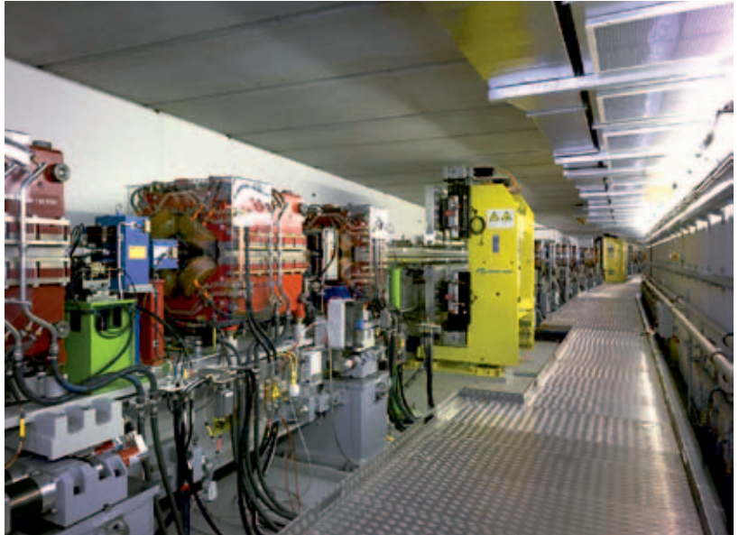
View along the storage ring PETRA III with bending magnets (blue), focusing magnets (red) and undulators (yellow) in the range of the photon experimental hall.
