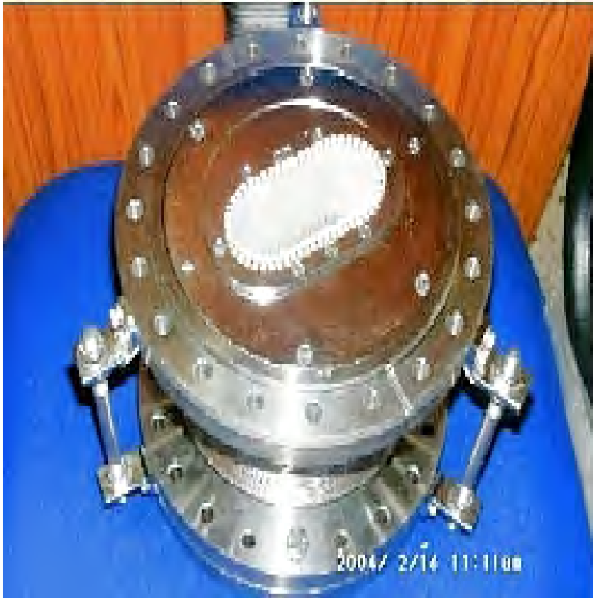
A RF-shielded Bellow Assembly
