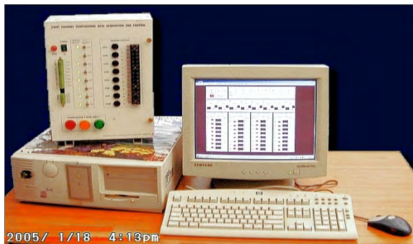
Eight-Channel Temperature controller unit.
