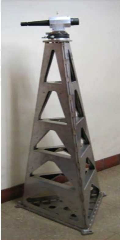
Optical Lever Transmitter on Pylon
